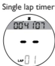
Press [S/S], the timer will stop, “01” will keep flashing. The single lap time length is recorded.
