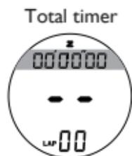
When the screen is in “all zero”, press [S/S] to start recording.
